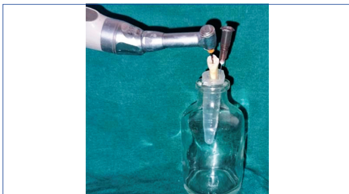
[Table/Fig-4]: Modified Myers and Montgomery debris collection apparatus assembled using a pre-weighed 1.5 mL Eppendorf tube supported within an empty Local Anaesthetic (LA) glass vial. Apically extruded debris was collected in the Eppendorf tube during root canal instrumentation.
